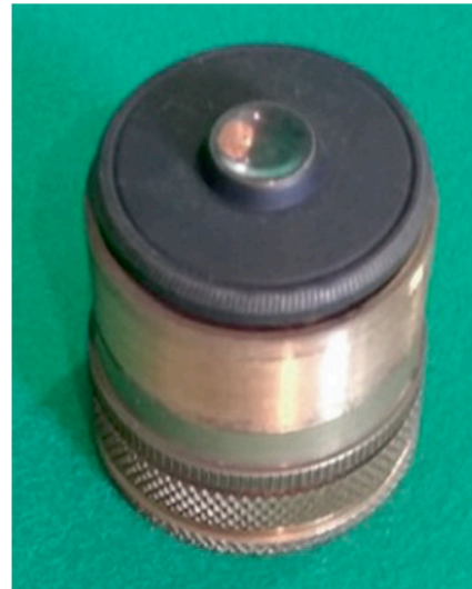
Fig. 26.5 Fabry photometer baseplate without plateholder. The filter, Fabry lens and aperture screwed into the central hole. SAAO Museum Inv. M046, part. (Photo: ISG)
