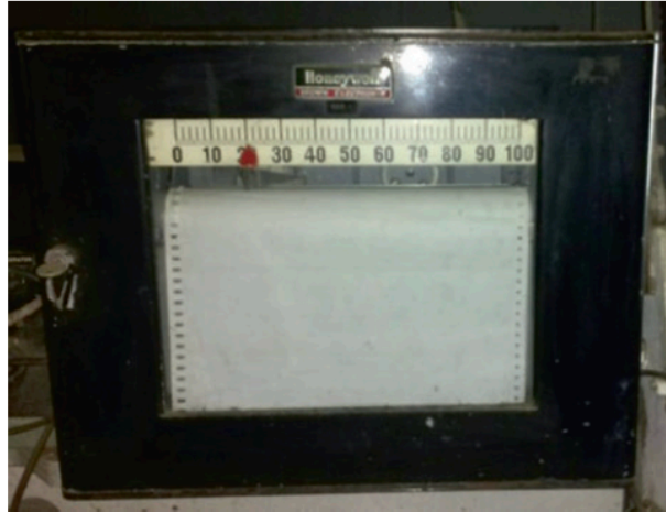
Fig. 26.16 One of the Honeywell-Brown instruments that were the primary recording medium for all of Cousins later photometry. The scale was accurate to one part in 1000. (Photo: ISG)
