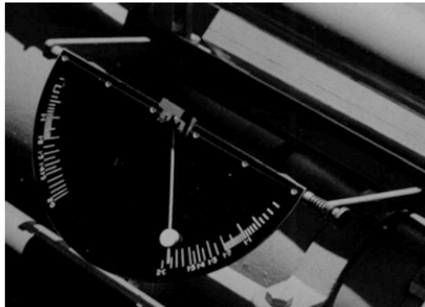
Fig. 26.8 Cousins Airmass Indicator. The axis was mounted parallel to the tube of the telescope and the scale stayed in a vertical plane (SAAO Archives P3571)
