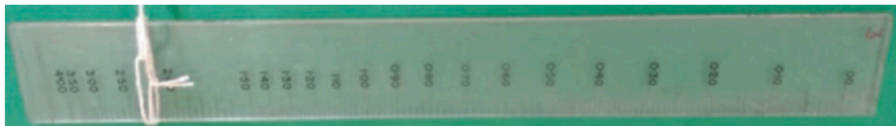
Fig. 26.17 Magnitude ruler used by Cousins for reading the Brown recorder charts. To obtain maximum accuracy, the deflection on the chart was kept as high as possible (SAAO Museum Inv. M108)
