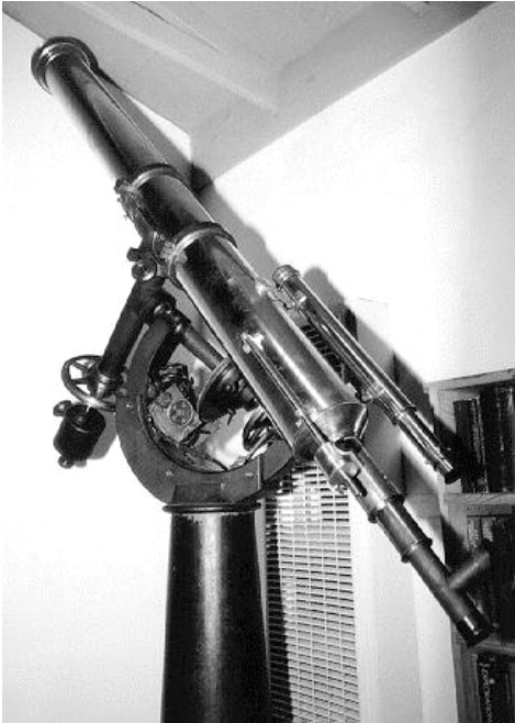
Figure 10. This 5-inch refractor from the private collection of John Briggs is a perfect twin to the original eight ‘USNO, Transit of Venus telescopes’ made by Alvan Clark & Sons, complete with their unmistakable signature wrapped around the tailpiece (Warner & Ariail 1985). Although this telescope is dated 1875 (the USNO Transit of Venus telescopes were all dated 1874) it bears no serial number and instead carries the beautifully hand-painted words ‘Abbot Female Academy’ on an iron casting inside the transportable pillar. Briggs traced the history of this telescope, verifying it being a ninth USNO Transit of Venus telescope, made by the Clarks, presumably as a backup in case something happened to one of the original eight. He found some surviving correspondence about the early plans for a telescope at Abbot Academy where the school originally envisioning another Clark telescope (a 7½-inch) which evidently they never got. It seems as though another telescope became available instead (this 5-inch) and after some challenging fundraising, they snapped it up.
