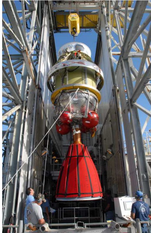
December 2008: On Complex 17-B at Cape Canaveral Air Force Station in Florida, the second stage of the Delta 2 rocket for the launch of NASA's Kepler spacecraft is moved inside the mobile service tower. Details: http://mediaarchive.ksc.nasa.gov/detail.cfm?mediaid=38875
