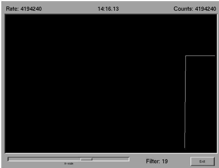
Figure 2: The XLUCY monitor form. This displays the count rate in graphical form.
