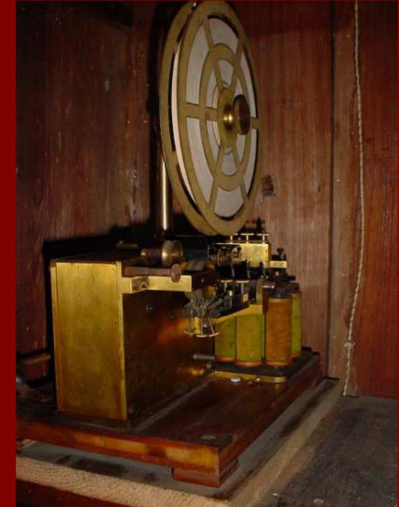
The CHRONOGRAPH was similar to a Morse code printer. The observer pressed a key to record a precise time next to ticks from a master clock.
