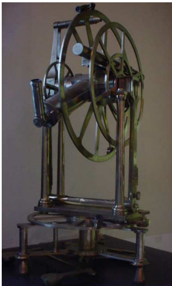
Figure 9: Dollond repeating transit used by the first HM Astronomer at the Cape, Rev Fearon Fallows, before the Royal Observatory building was completed.
