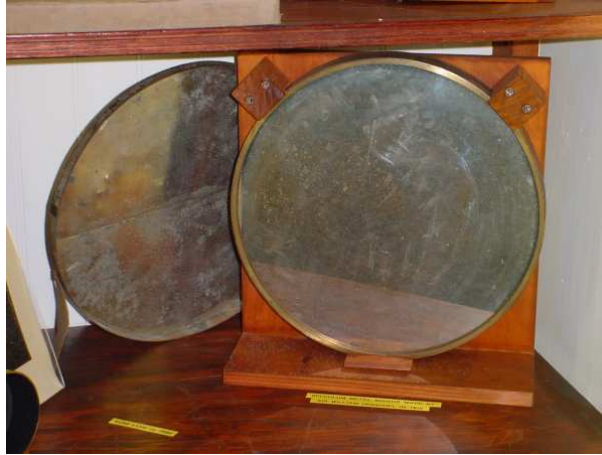
Figure 10: Speculum metal telescope mirror ground by William Herschel, 1811.
