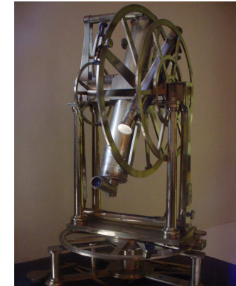
A "Repeating Transit" by Dollond of London (1819). Used by the first HM Astronomer, Fearon Fallows, for determining star and planet positions before the main building was finished.
