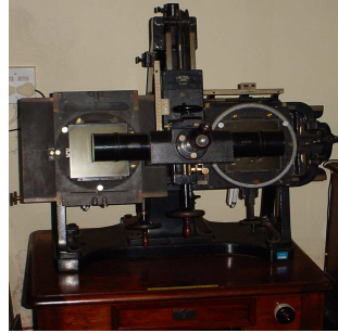
Model of the 74-inch (1.9m) Radcliffe telescope, now in Sutherland, made by Grubb Parsons of Newcastle, UK, in the early 1930s. The telescope was completed in 1948.
