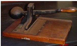
Early multi-hole punch, believed to have been designed by G.B. Airy, Astronomer Royal at Greenwich.
