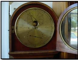
The observer needed to count the loud ticks of the clock as he watched the star cross a fine wire in the eyepiece. Afterwards he looked at the clock and wrote down the sidereal time.
