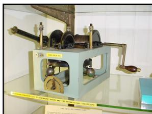
Small drive clock from the 6-inch telescope (weight not shown).
