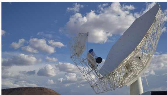
Fig 3. A single MeerKAT antenna. The configuration is an offset Gregorian. The radio signals bounce off the big dish onto the smaller one and then into the receiver just below the small one. Two receivers can be seen on the turntable.
