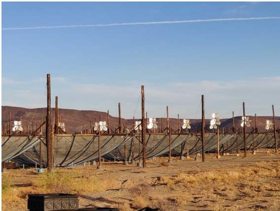
Fig 5. Side view of the HERA array. The dish surface is constructed of wire birdcage netting and supported by ordinary PVC tubing and fittings.
