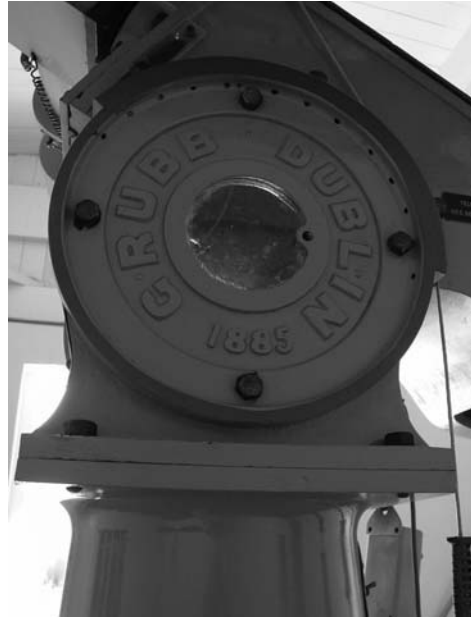
Figure 19. The mountings of the original 6-inch 'Transit of Venus' telescopes were made to be portable but were found to be very unstable. After numerous complaints by Gill, Grubb later replaced it with a mounting designed for an 8-inch telescope, as can be seen from the date on the mount.
