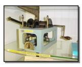
Small drive clock from the 6-inch telescope (weight not shown).
