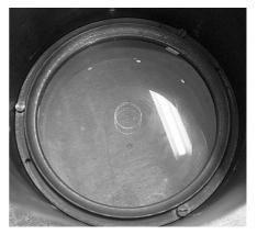
Figure 6 The objective lens of the 7-inch Merz. Unfortunately some damage in the centre of the front surface is visible, probably caused by a badly fitting lens cap. One of the postage stamp stub separators can be seen at the top right.
