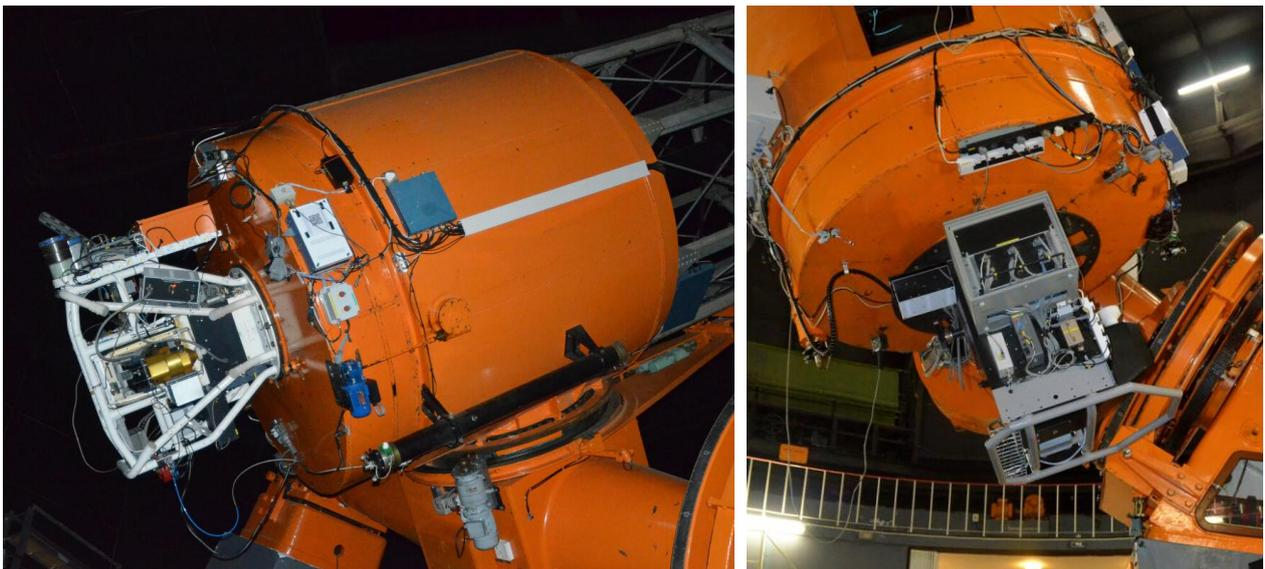
Figure 1. The old Cassegrain Spectrograph (aka Cassie) on the 74-inch telescope (left) and the upgraded instrument (SpUpNIC) shortly after installation in October 2015 (right).
