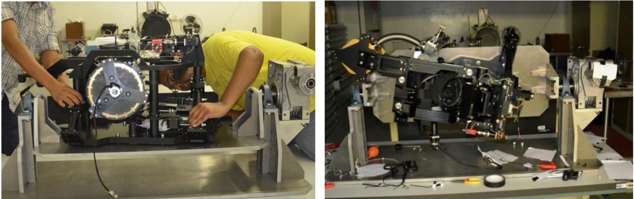
Figure 15. Bolting the instrument to the alignment jig (left) required everything to be upside down, but the alignment process was done with the jig rotated through 90° and then securely locked in that position (right).
