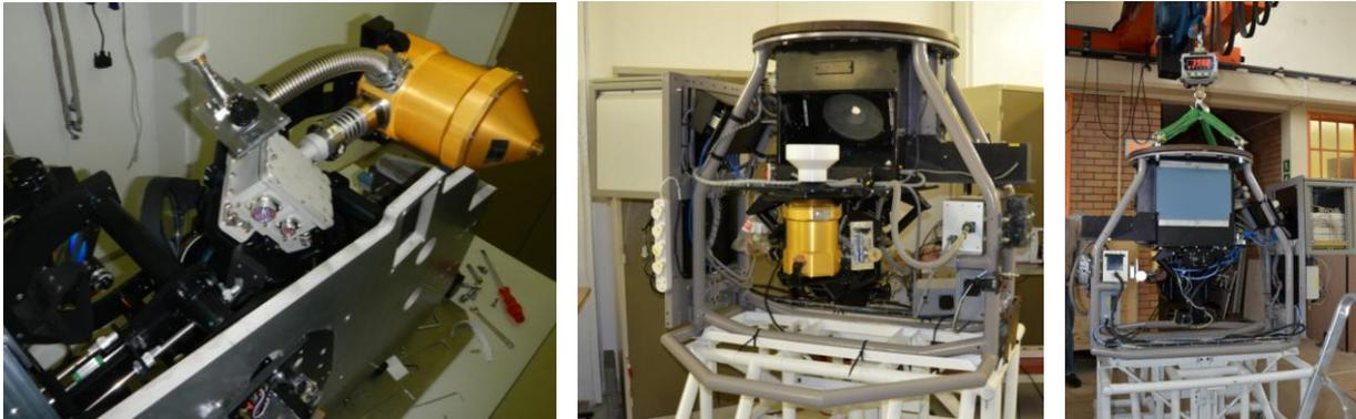
Figure 19. The cryostat connected to the rest of the lower box (left), the lower box attached to the upper box (centre) and the largely complete assembly weighing in at approximately 400 kg (right).
