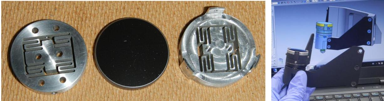
Figure 10. The collimator secondary mirror and wire-cut flexure mounts for decentre adjustment (left) and the complete assembly that includes tip/tilt and focus adjustability (right).
