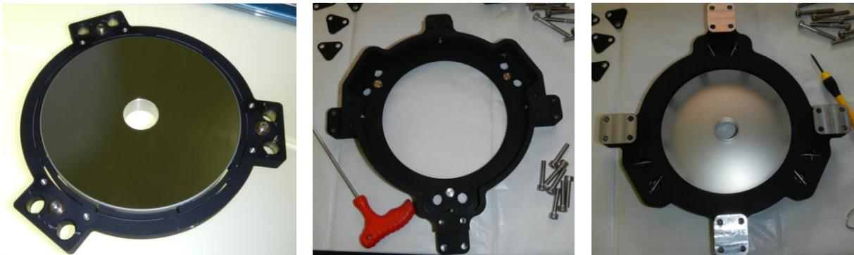
Figure 11. The collimator primary mirror bonded into its radial flexure (left) and the mirror cell with its pairs of decentre adjusters and the three tip/tilt adjusters that also provide focus travel (centre). The assembly is held together by three pairs of spring hooks with dowels locking each end. The grey patches of epoxy are visible through the back of the mirror (right).
