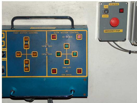
Figure 8.6: Blue telescope control console with “Emergency Stop” box.
