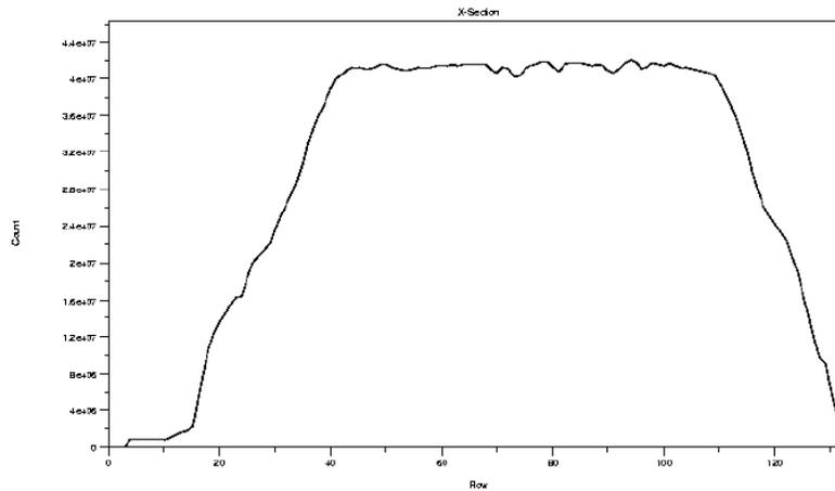
Figure 7.9: A cross section of a (grating 7) flat field.
