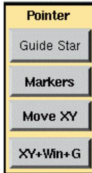
Figure 7.17: Use the **Move XY** option to move a star to the centre of the field and **Guide Star** to mark the selected guide star.
