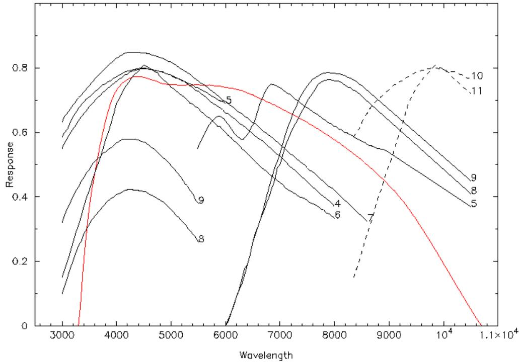
Figure 9.15: Grating efficiencies. Note that some grating efficiencies are displayed for both first and second order. The red line indicates an illustrative efficiency for the CCD detector.
