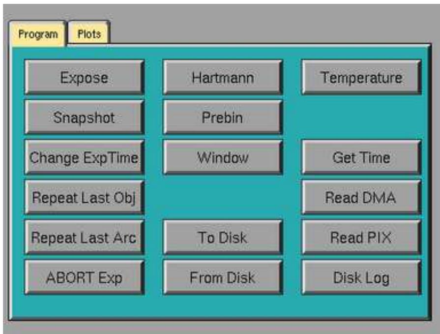
Figure 6.4: The spectrograph control program – Control Panel
