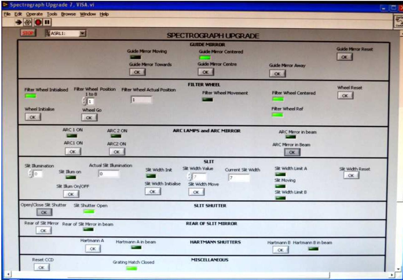
Figure 4.1: The LabView Spectrograph Control Panel GUI.
