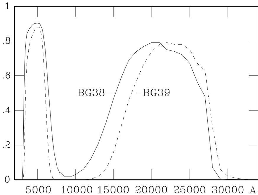
Figure 9.18: Representative transmission functions for Schott BG38 (solid line) and BG39 (broken line) glasses (1mm thickness) over a much larger wavelength range.
