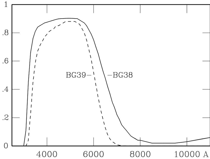
Figure 9.17: Representative transmission functions for Schott BG38 (solid line) and BG39 (broken line) glasses (1mm thickness). Note the “red leak” and the fact that BG39 suppresses red light more effectively than BG38.
