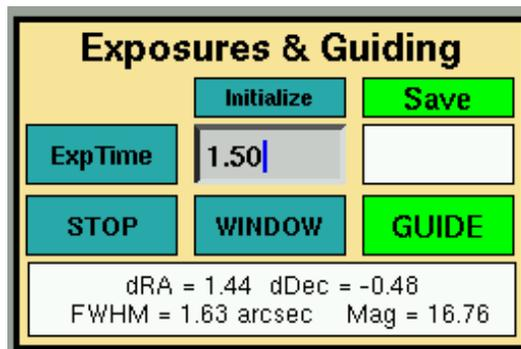
Figure 7.18: Exposures & Guiding panel. **Guide** is green when guiding; red when not.
