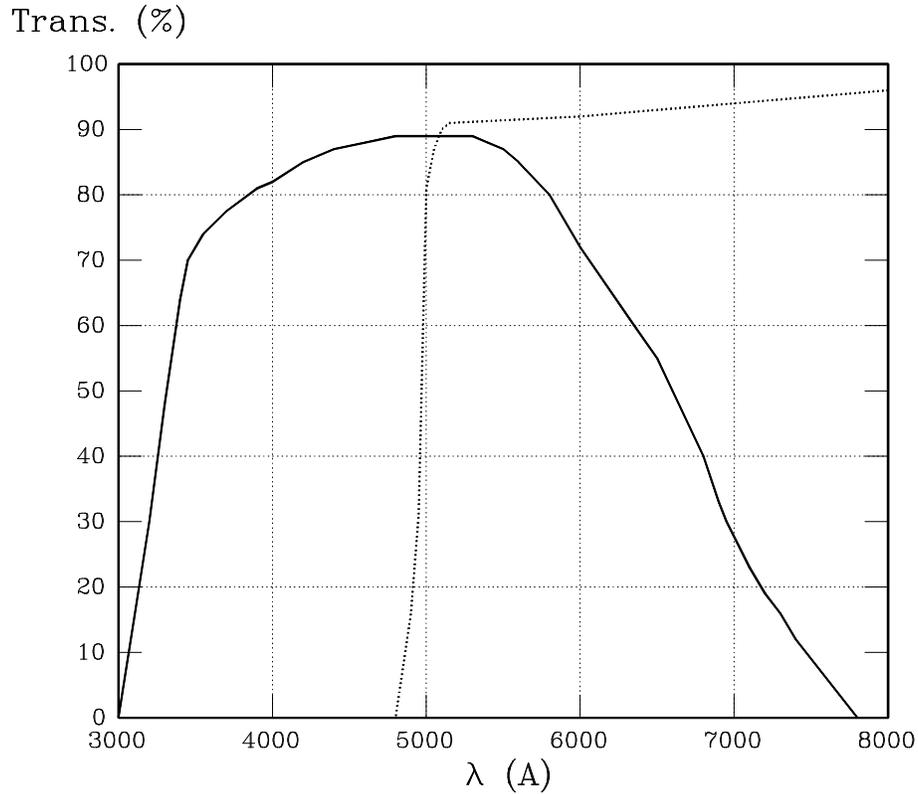
Figure 9.16: Approximate transmission curves for the BG39 (solid line) and GG495 (broken line) filters.
