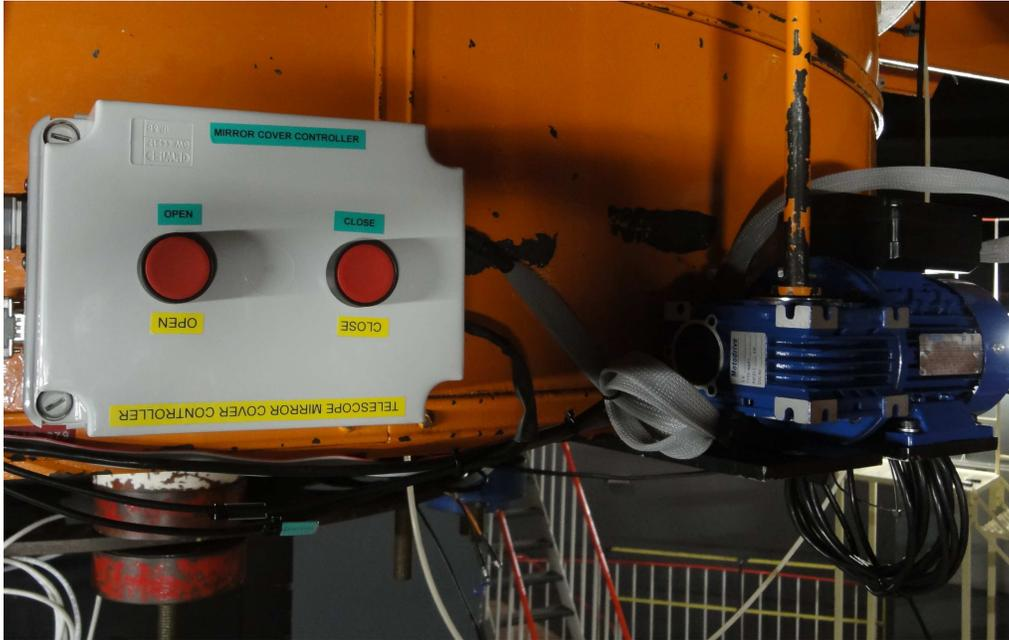
Figure 7.7: The Mirror Cover Controller box, located on the north side of the primary mirror cell.
