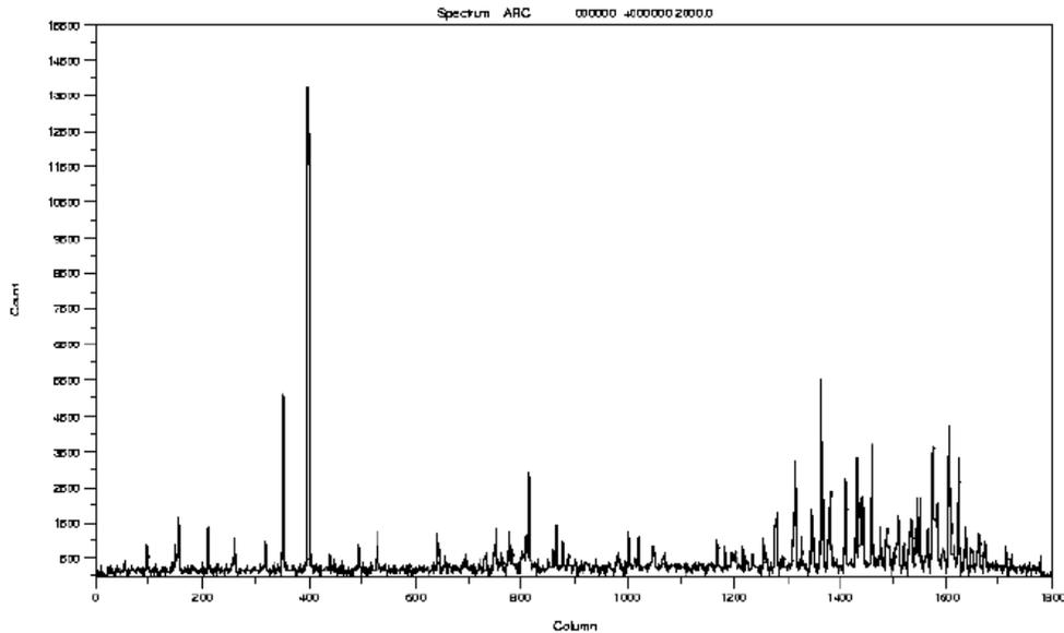
Figure 3.7: Grating 7 Cu-Ar arc (grating angle  $17^\circ$ ; central wavelength  $\sim 5900\text{\AA}$ ; BG38 filter).
