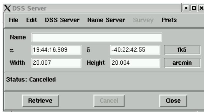
Figure 7.3: The DSS Server under DS9. Note - the default height and width for the 1.9m telescope is 10, not 20.
