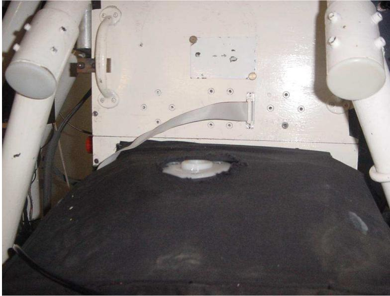
Figure 3.8: Dewar refill hole (white nylon ring)
