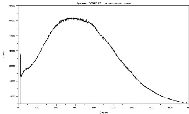
Figure 7.10: A sample grating 7 flat field. Note the rapid fall off in flux towards the blue end (right in this case). Flats obtained in the red will tend to be much flatter – and especially if they span a smaller wavelength range.
