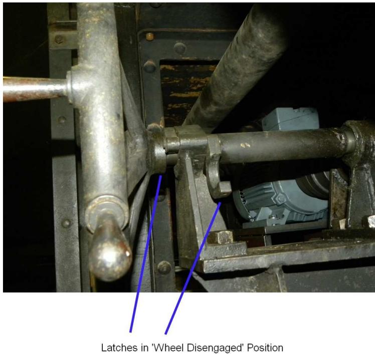
Figure 8.3: Manual shutter control wheel in disengaged position.
