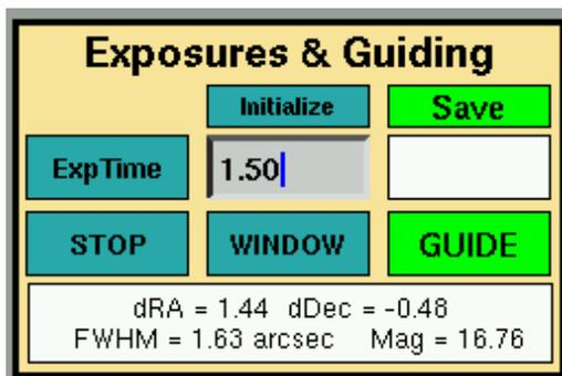
Figure 5.7: The Exposures & Guiding panel of the TCS. **Initialise** allows resetting of the Merlin crate.
