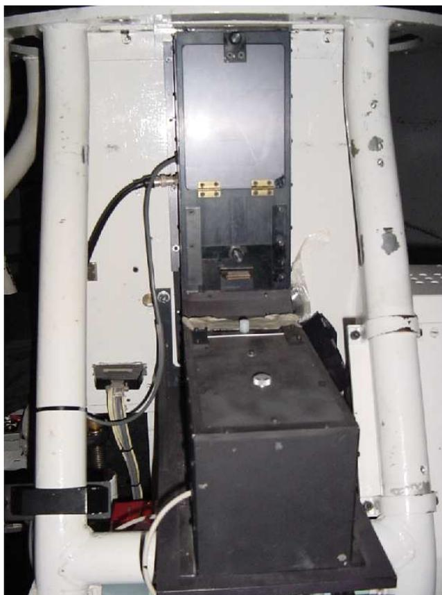
Figure 3.5: West side of the spectrograph. The arc lamp unit is near top, centre. Just above the centre of the picture is the filter unit for the arc beam.
