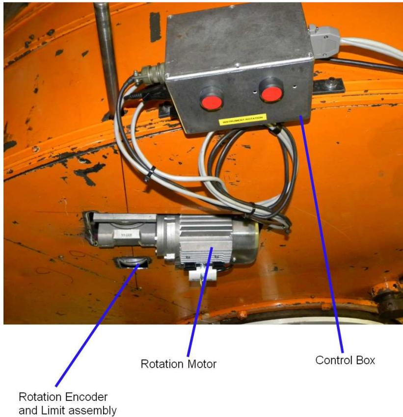
Figure 3.9: Instrument angle setting unit.
