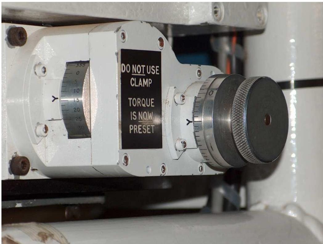
Figure 3.2: Grating angle setting unit.
