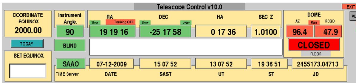
Figure 5.2: Telescope and dome status information is given in the top portion of the TCS software display.
