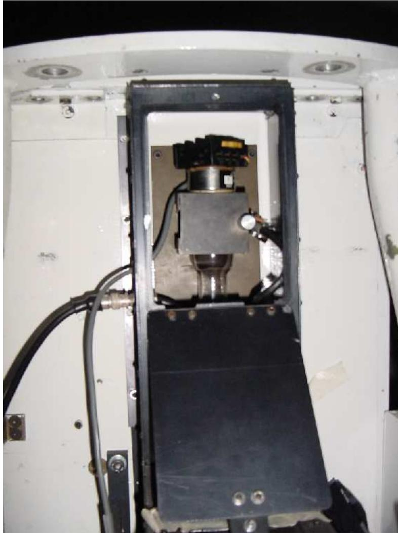
Figure 3.6: Close up of the arc lamp unit with the hatch folded down. The small retaining “gate” for the arc lamp and the lamp itself (with socket at the top) can be seen.
