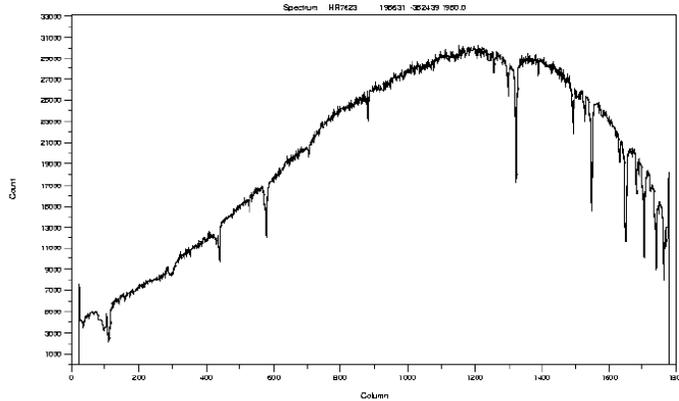
Figure 7.20: Spectrum of a bright B2IV star (HR7623). This was a 4-second exposure taken with grating 7 (angle  $17^\circ$ ; centred near  $5700\text{\AA}$ ). Balmer series lines are obvious with atmospheric bands at the left (red) end.
