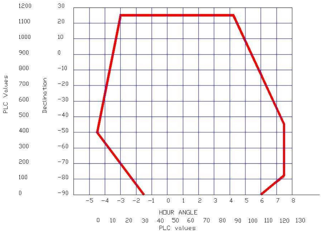
Figure 2.7: Telescope limits. The red line indicates where the telescope reaches software limits and stops.
