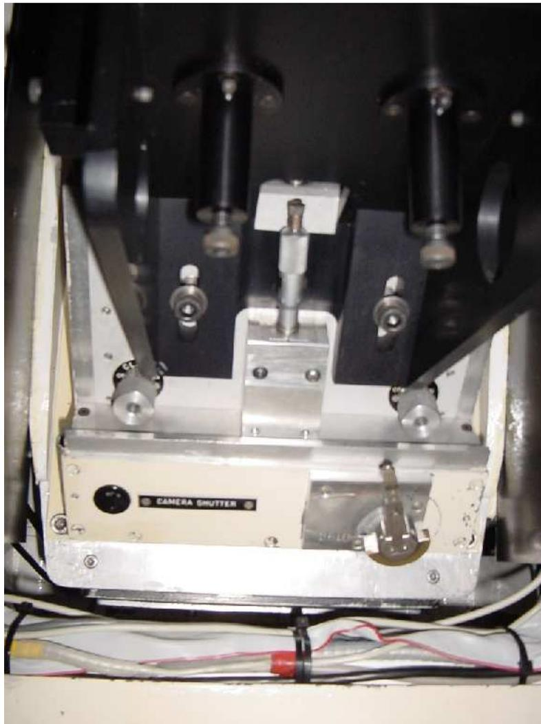
Figure 7.4: The back of the spectrograph with the black cloth “box” removed. The micrometer unit for setting the spectrograph focus is central; just below it, to left and right, are the two knurled cylindrical clamps. Just below the right-hand clamp is the lever that opens and closes the camera shutter.
