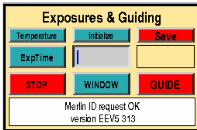
Figure 7.11: The Exposures & Guiding panel of the TCS.  – or just typing in a different time – will change the A/G exposure time.
