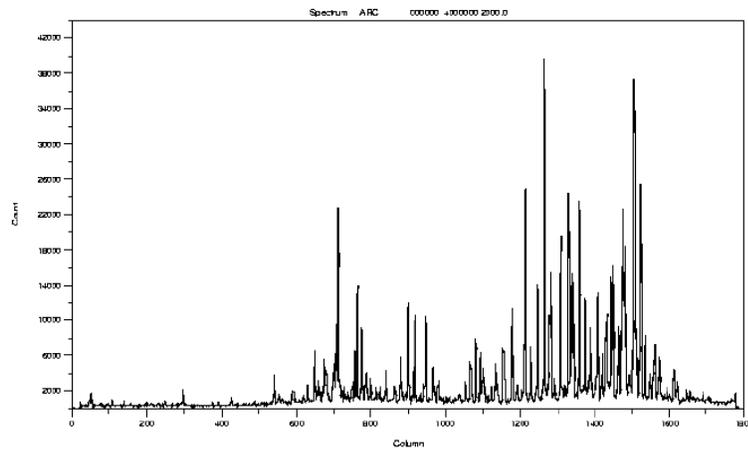
Figure 9.7: CuAr arc for grating 7 (angle  $17.2^\circ$ ;  $\lambda_c \approx 5700\text{\AA}$ ) with a BG39 filter in the **arc** beam. Note the almost total disappearance of the red lines (and the scale difference)
