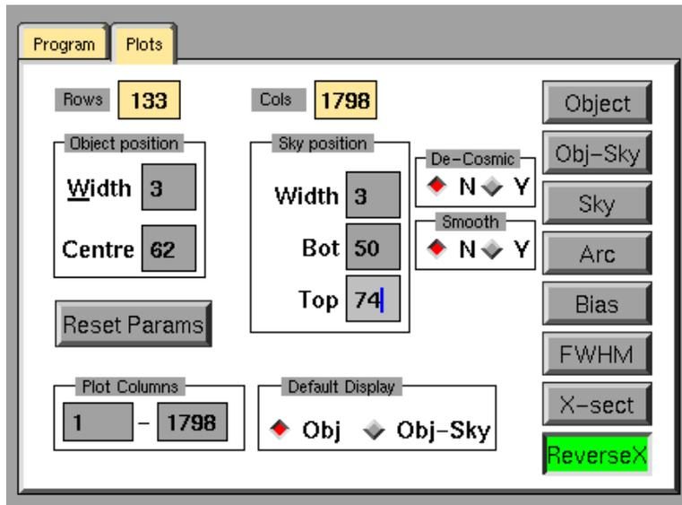
Figure 7.19: The **Plots** panel of **RunSpect**. In the figure, **ReverseX** is clicked which will put the blue end of the spectrum displayed on the left of the display panel.
