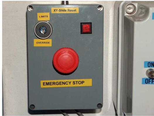
Figure 8.7: Close-up of “Emergency Stop” box.
