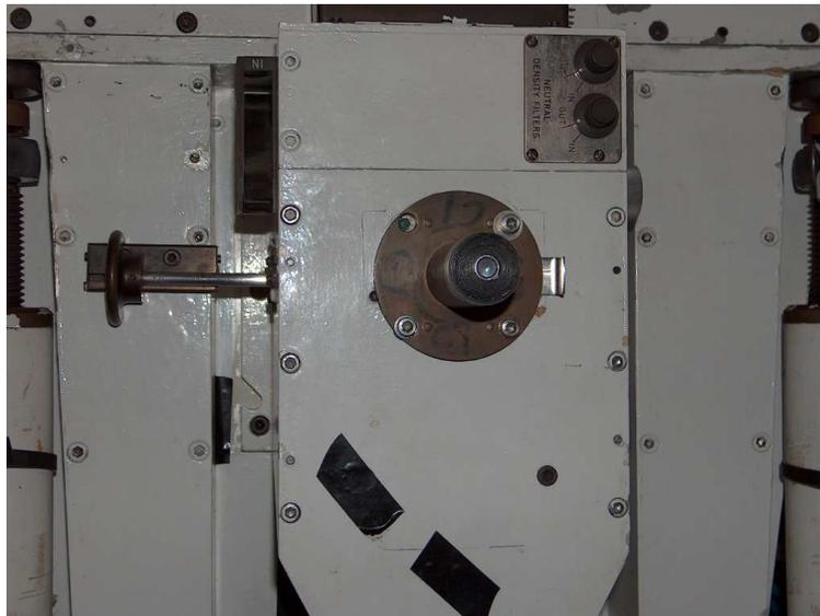
Figure 7.15: Rear-of-slit viewing eyepiece.
