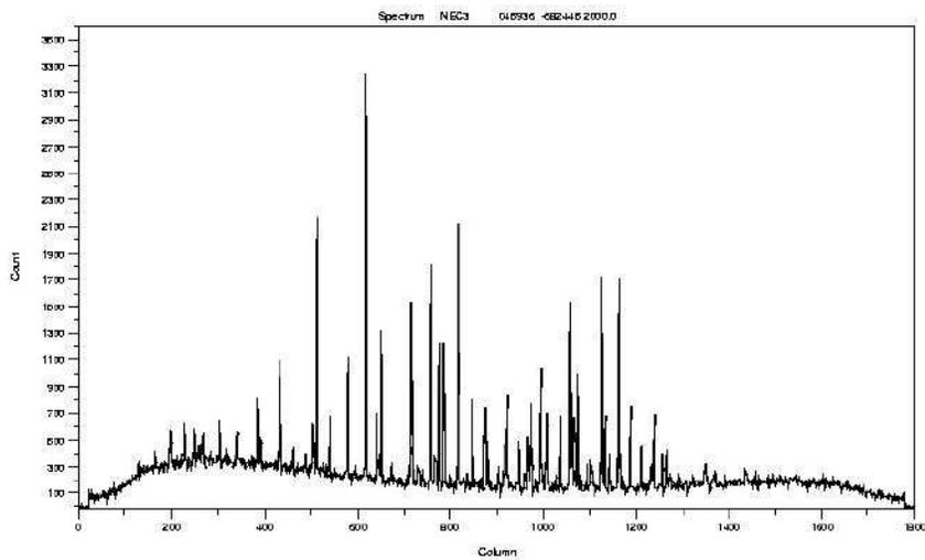
Figure 8.8: Grating 6 arc (range about 3600 – 5200 Å). Note the underlying background “bumps” caused by the light at the top of the stairwell.
