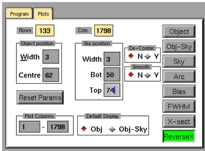
Figure 7.8: The **Plots** panel of **RunSpect**. Note, in this example **ReverseX** has been clicked; blue will be on the left in the spectrum display. Also, three rows (“width”) will be displayed.
