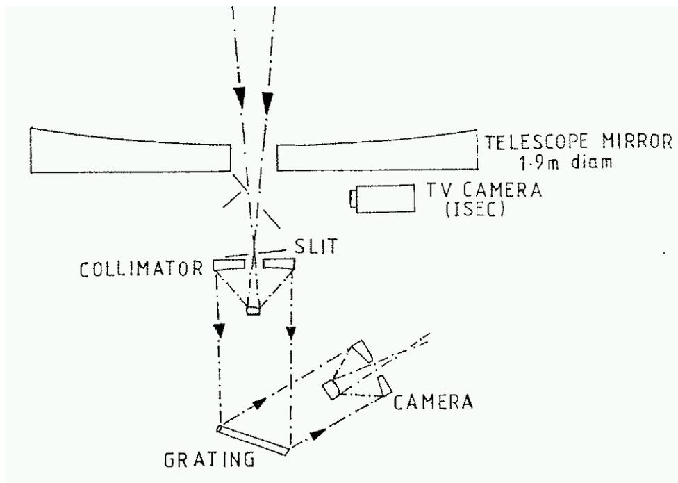
Figure 3.1: Sketch of the basic elements in the spectrograph. Note that a CCD now replaces the “TV Camera” on the xy slides.
