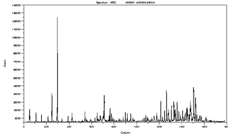
Figure 9.6: CuAr arc for grating 7 (angle  $17.2^\circ$ ;  $\lambda_c \approx 5700\text{\AA}$ ) with a BG38 filter in the **arc** beam.
