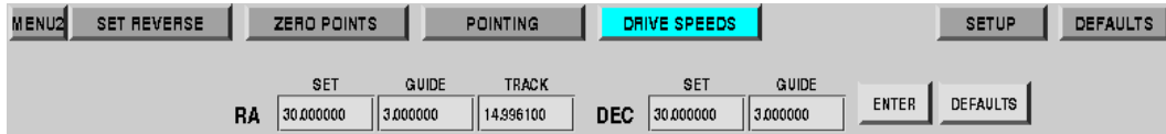
Figure 8: Adjustments to RA & Dec motion can be made using the DRIVE SPEEDS button.
