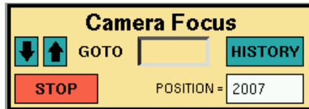
Figure 16: The A/G “Camera Focus” panel. The telescope should be focussed using the science detector before adjusting the A/G camera focus.
