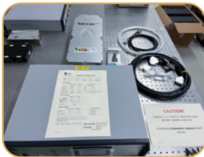
Figure 1. The 800 nm Ti:Sapphire femtosecond pulsed laser system that will drive the LFC.
