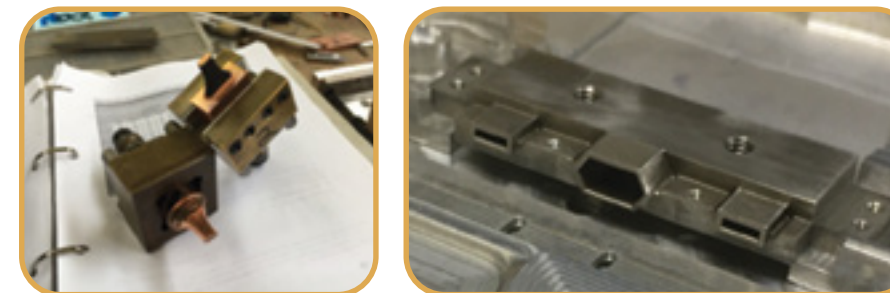
Figure 4. At left are the final set of 'positive' electrodes for the 'large aperture' IFU mounts for the SALT slit-mask IFU. The final article, made in stainless steel is at the right, shown in a test-fit inside the cassette that will hold the IFU, before inserting fibre-optics.
