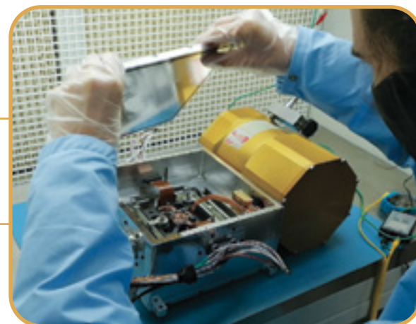
Figure 2. Final assembly of the test cryostat with a 6k x 6k engineering sample chip installed, allowing the development team to test various other aspects of the system on a representative CCD.
