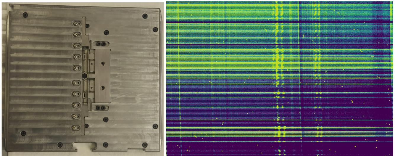
**Figure: Left: The fully assembled SMI-200 instrument. Right: Spectra of a star-forming galaxy through several fibers of SMI (each individual horizontal trace is spectra from a fiber). The vertically misaligned zig zag blobs are Hydrogen-alpha (brightest), doubly ionized Nitrogen and Sulphur emission lines.**
