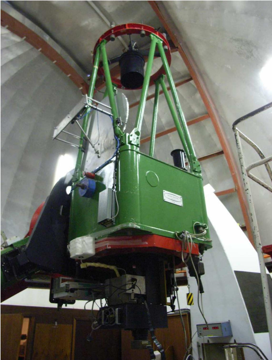
Figure 1: The 0.75m telescope with the UCT CCD mounted below it.
