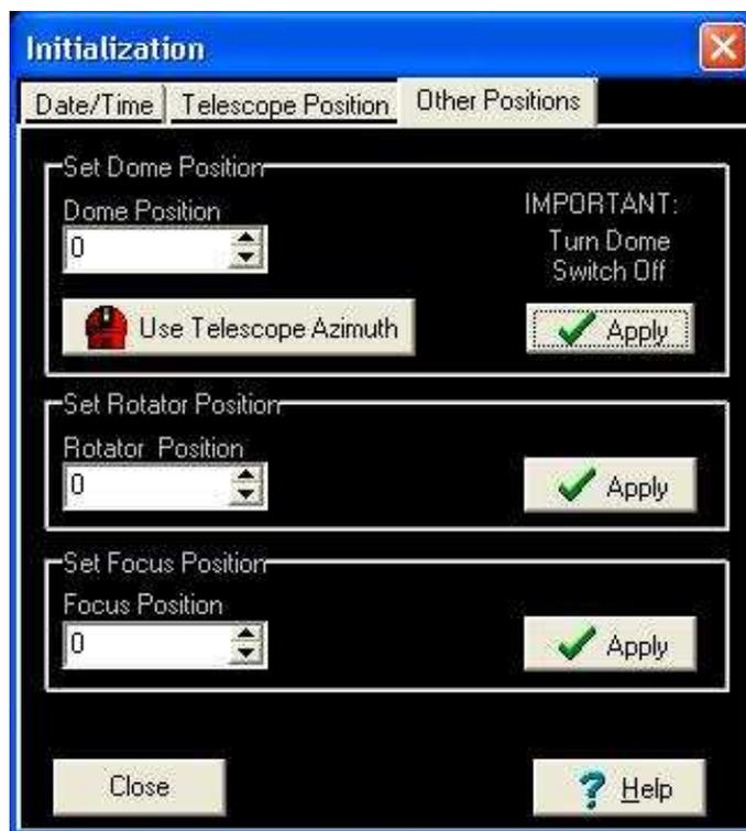
Figure 4.1: Re-initialising the dome position under the Initialisation screen.
