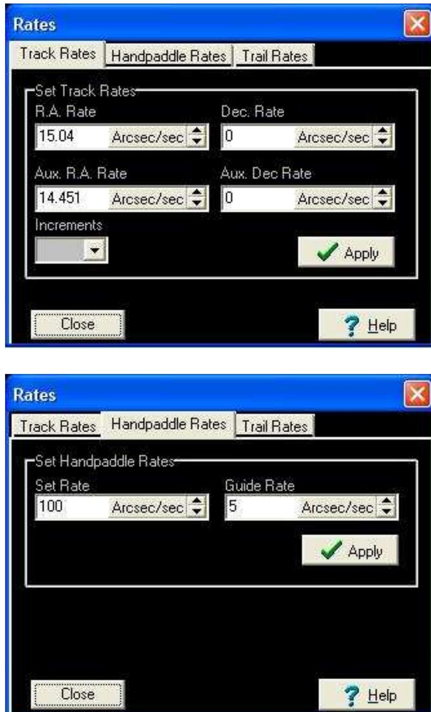
Figure 2.8: Adjusting telescope track rates (top) and handpaddle rates (bottom).
