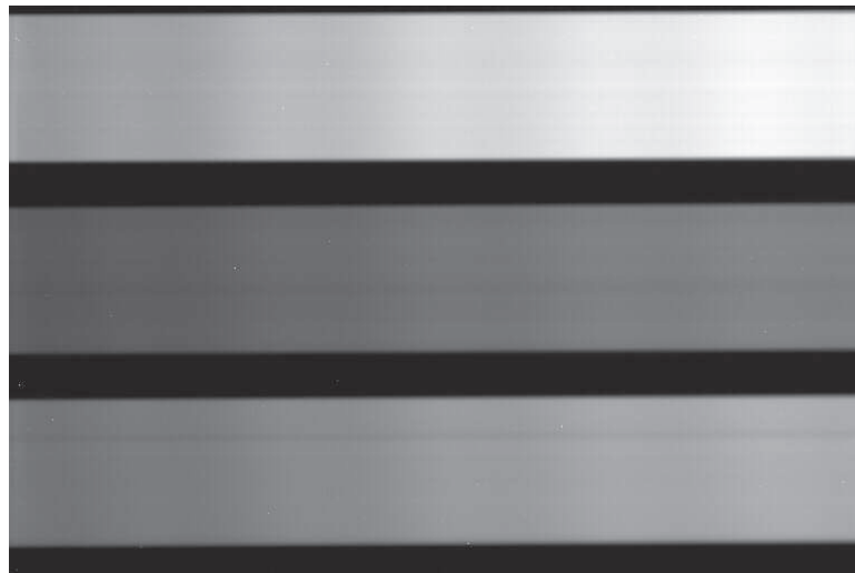
Figure 2.10: A two dimensional not yet reduced flat field image. Taken with the 900-line grating and an exposure time of 600s. The three slits can be seen. The illumination of the slits is different because of the different slit sizes. The periodic change of the amplitude is also visible with a period that is the same for all three slits. The period changes with the thickness of the glass plate that protects the CCD chip ( http://www.astrosurf.com/aras/fringing/schlatter/ripple.htm , accessed on August 29., 2011).
