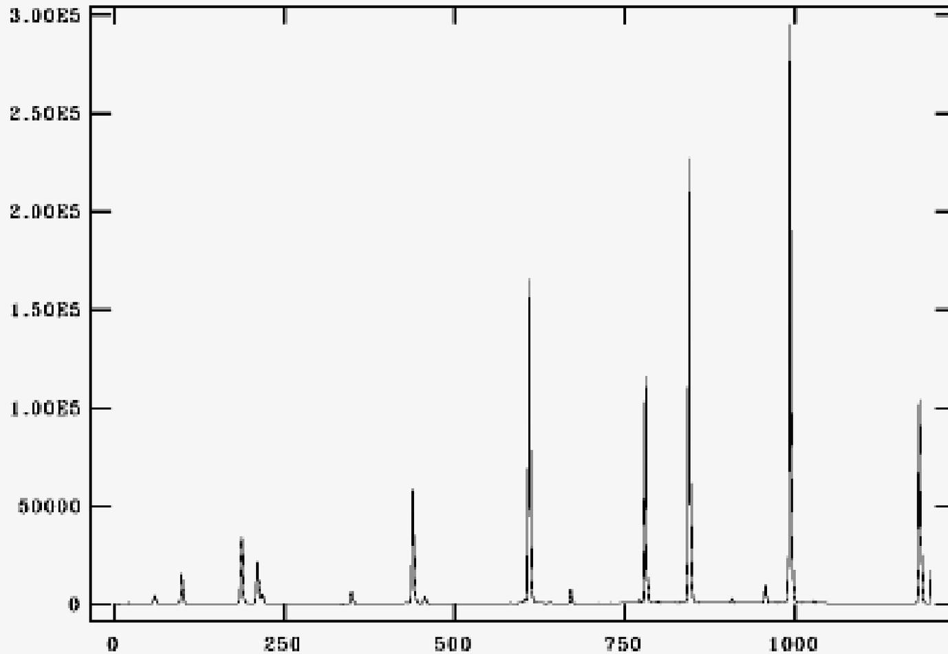
Sometimes fit a master arc taken in the afternoon and use arcs taken adjacent to program objects to make a zeropoint shift to the wavelength solution.
