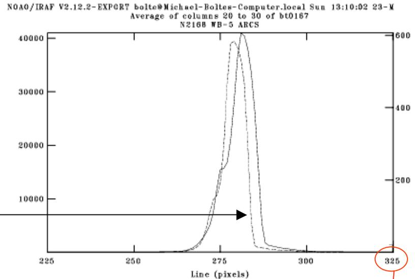
Two lamp spectra from LRIS taken at different telescope positions
