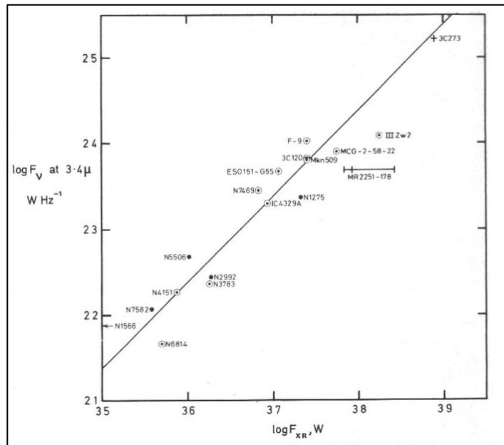
One of the most interesting conclusions of this paper was that the X-ray flux in the 2-18 keV range was well correlated with the L-band (3.4 micrometers) flux. This was a confirmation of some earlier work by Elvis et al *MNRAS* **183**, 129, 1978 and showed that the mechanisms involved had to be closely related.
