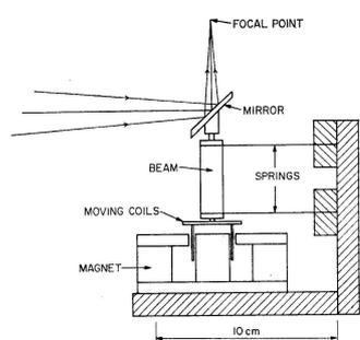
*Fig: Stepwise oscillating chopper. The springs could be adjusted so that the mirror moved strictly parallel to itself so that the detector always saw precisely the same pupil.*
