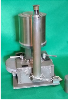
Fig 27. Photometer labelled “RP3 Photometer VI 1956 L.C.B.” [Laurie Brown]. Probably the photometer constructed for the 18-inch telescope. SAAO Museum Inv. M127 (Photo: ISG).
