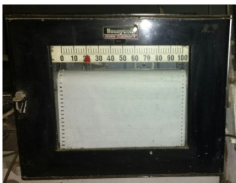
Fig 16. One of the Honeywell-Brown instruments that were the primary recording medium for all of Cousins later photometry. The scale was accurate to one part in 1000 (Photo: ISG).
