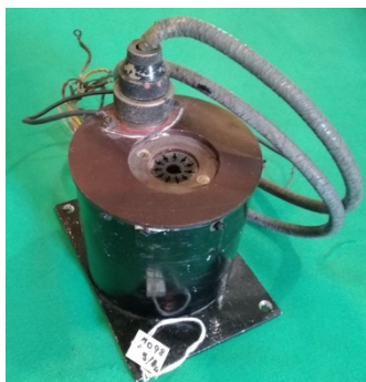
Fig 13. The separate voltage divider unit used with Cousin's early photoelectric photometers. This provided the correct voltage for each dynode of the photomultiplier. It was normally mounted on the telescope near the photometer. In later instruments the divider resistors were mounted behind the photomultiplier (SAAO Museum Inv. M098/3) (Photo ISG).
