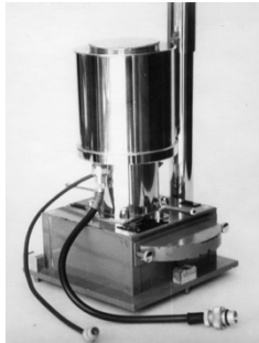
Fig 25. A Cousins photometer of the 2 nd type, EMI version that made use of the end-window EMI phototubes. Two of these photometers still exist. They continued to be used by Cousins for many years (SAAO Photo: P7581).
