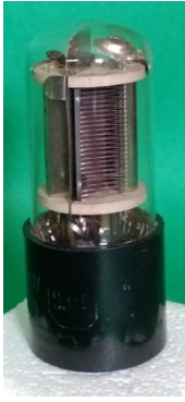
Fig 9. A “Side-View” Photomultiplier, the RCA 931A. Its black base indicates that this example was manufactured early on.
