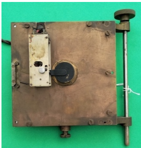
Fig 7. The rear of a plateholder showing the electromechanical shutter, a Fabry lens unit and (in this example) the hinge for swinging the whole photometer out of the way. SAAO Museum Inv. M046, part (Photo: ISG)
