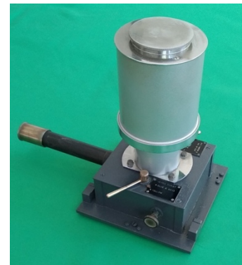
Fig 21. The first of the end-window versions of the photometer, using the lower part of the side-window version. SAAO Museum Inv. M253 (Photo: ISG).
