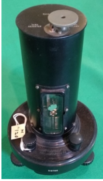
Fig 14. A Mirror galvanometer by Leeds & Northrup. These were the most sensitive type of moving-coil meter and were used to measure photocurrents before the advent of D.C. amplifiers using valves. A mirror was suspended on a very fine wire or quartz thread that supported the moving coil. It reflected a light beam that projected a dot on a distant scale. SAAO Museum Inv. M120 (Photo ISG).
