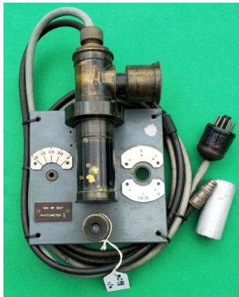
Fig 20. The upper part of the first version of the second photometer as it exists today. It was labelled "Photometer II". The filter and aperture levers were re-used on the next version. SAAO Museum Inv. No. M098/1 (Photo: ISG).
