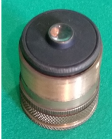
Fig 6. Example of unit containing Fabry lens, aperture and filter that was attached to the rear of the baseplate. SAAO Museum Inv. M046, part (Photo: ISG)
