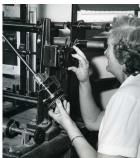
Fig 1. A Lady Computer measuring images with a Schilt microphotometer. On top right is the screen for the reflected beam from the mirror galvanometer that displayed the photocurrent from a detector (SAAO Archives P7963).
