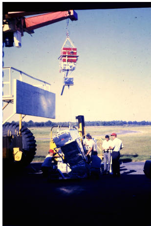
Fig 12: The gondola was covered with insulation and reflective foil. It is suspended from a line twister and above it is a chute for lead shot from the red ballast container. The red arms at the top of the launcher swing open to let the gondola float away as soon as the balloon has taken the load.
