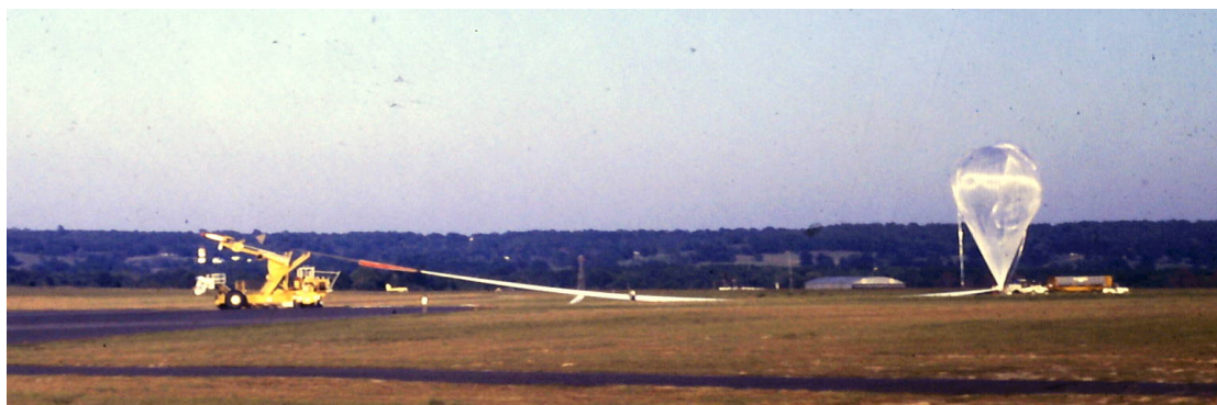
Fig 12: The gondola was covered with insulation and reflective foil. It is suspended from a line twister and above it is a chute for lead shot from the red ballast container. The red arms at the top of the launcher swing open to let the gondola float away as soon as the balloon has taken the load.
