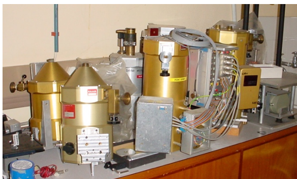
Fig 7. Dewar graveyard: Some of the camera and photometer cryostats that I designed, about the time I retired finally (2005).
