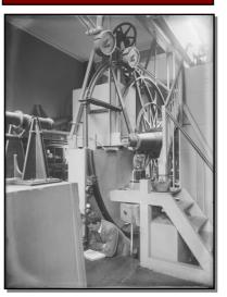
In 1855 a **Transit Circle** (above) designed by the Astronomer Royal at Greenwich, G.B. Airy, was acquired to take the place of both the Transit Telescope and the Mural Circle. One observer could now determine both Right Ascension and Declination. This was a copy of a similar instrument installed at Greenwich in 1851. The manufacturer was Ransomes and May, who usually built agricultural machinery!
