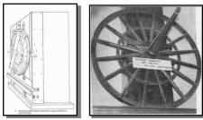
To measure the declination a large **Mural** (wall-mounted) **circle** with a telescope and six microscopes to read the scales were used.
