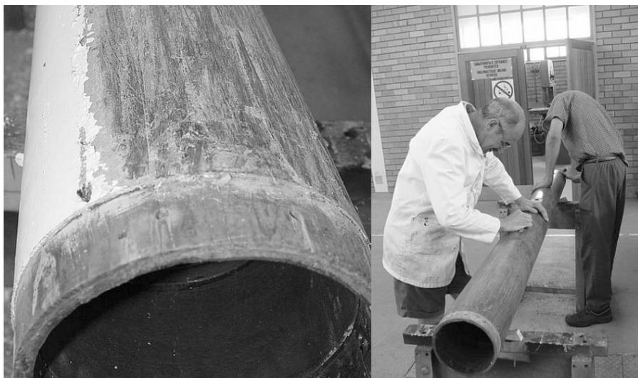
**Figure 7** After stripping off several layers of paint, Dougie Metcalfe (white coat) and Malcomb Henricks prepared the tube for varnishing. The construction of the tube is quite interesting with a lighter wood core, covered with mahogany veneer, probably all hand made. Take into consideration that the tube tapers down from front to back.
