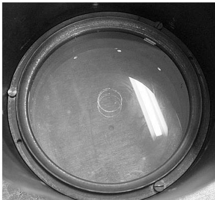
**Figure 6** The objective lens of the 7-inch Merz. Unfortunately some damage in the centre of the front surface is visible, probably caused by a badly fitting lens cap. One of the postage stamp stub separators can be seen at the top right.
